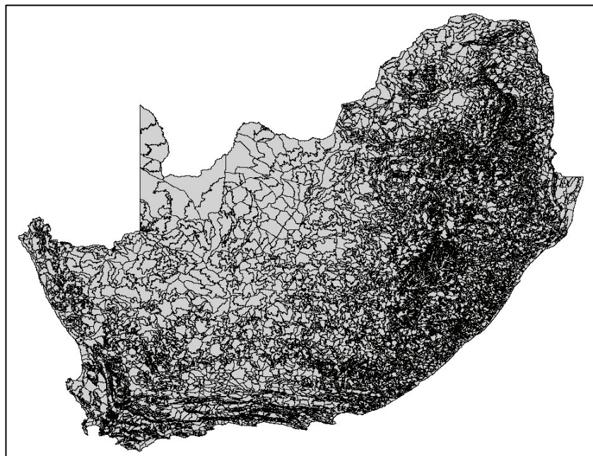
Figure 2.2.4 Delineation of the RSA, Lesotho and Swaziland into 5 838 hydrologically interlinked and cascading Quinary Catchments (Schulze and Horan, 2010)
